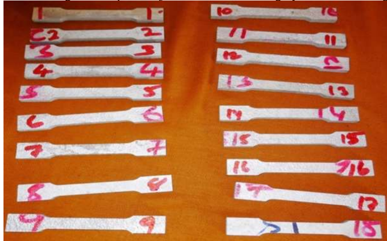
FIGURE 5. Tensile specimens made for the current investigation.
